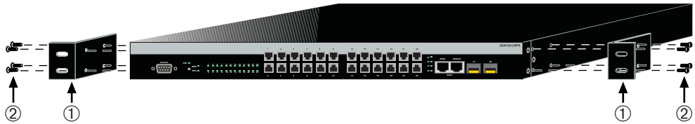
Figure 3-6 Attaching the Rackmount Brackets
